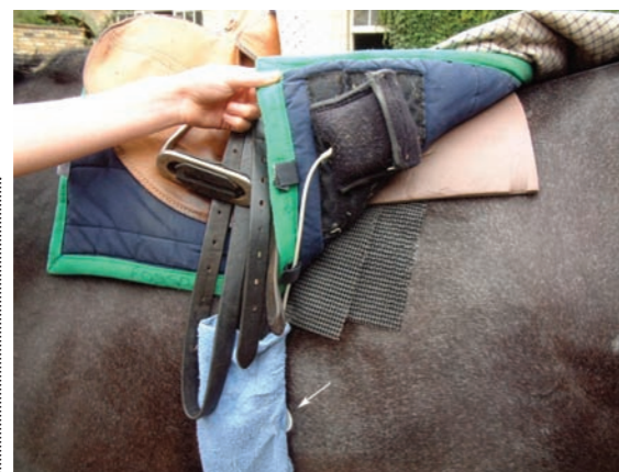
For an exercising ECG, a small monitor is attached to the tack, in this case with Velcro on a saddle pad, and electrodes are attached to the horse's surface. In this case, one of the electrodes is just visible under the girth (arrow); others are placed over the heart below this one and on the right side.
